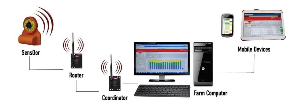
View of the structure of system, transmission routers and data analysis (Grodkowski et al., 2022).
